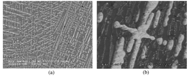
Fig. 2. SEM images of the crystalline Ni 42 Nb 28 Zr 25 Ta 5 membrane: (a) cross-sectional view and (b) cross-sectional view under higher magnification.
